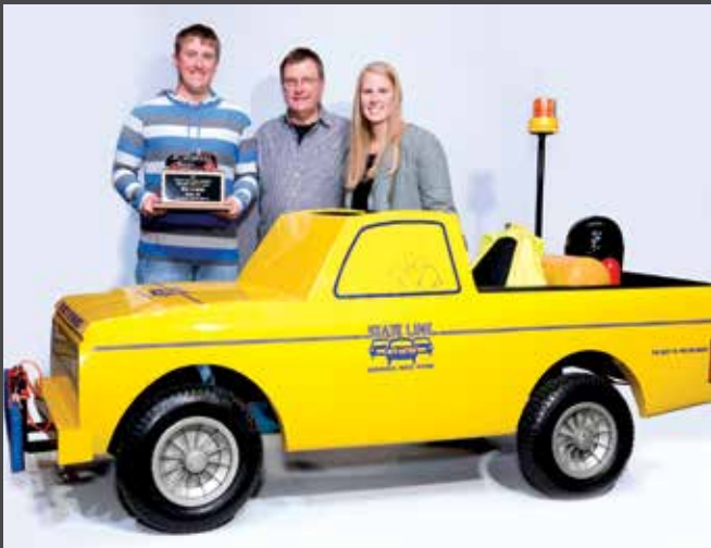
Stateline Auto Auction built a 2014 Jump Truck with custom steel, fabricated by Rob Bennett of Waverly, New York, and finished by State Line Body and Paint Shop. The team of John Williams, Chris Waters and Ed Garrity invested almost 130 hours in the construction, including accessorizing it with jumper cables, compressed air system, push bumper, beacon lights, trash receptacle, fire extinguisher and first aid kit. This car won "Best In Show."
